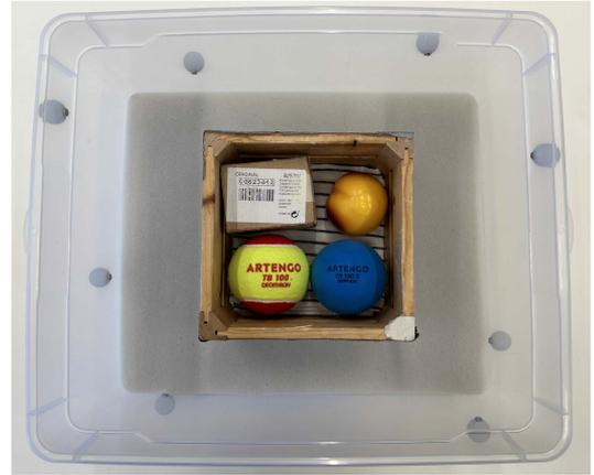
Fig. 17. Target box with two levels of error tolerance. Inner small box:  $15 \times 15$  cm. Outer large box:  $37 \times 33$  cm.
