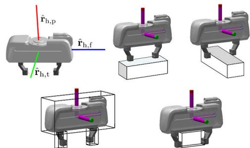
Fig. 16. Top: Definition of the local frame used to compute  $\mathbb{J}_a$  for the Panda Gripper and examples of alignment of the gripper with a box. Bottom left: approximation of the collision volume  $\mathcal{O}$  as union of three cuboids. Bottom right: fingers' closing region  $\mathcal{C}$ .
