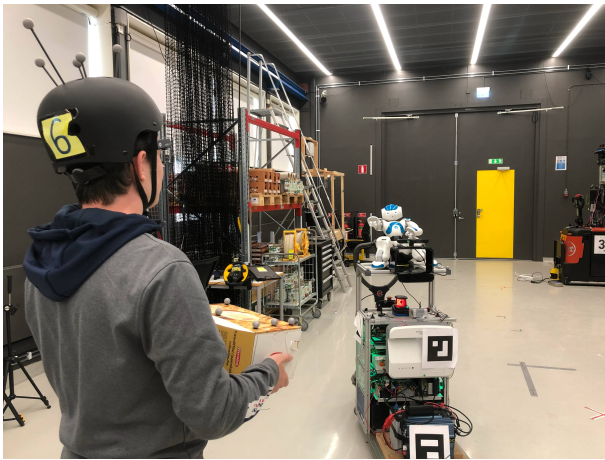
Fig. 2: In Experiment A, participants interact with a robotic forklift. The ARMoD instructs the participants to place an object on the forks of the mobile robot.
