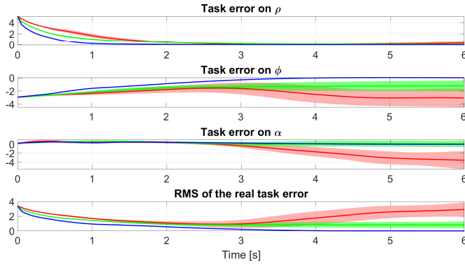
(b) The value of the mean RMS with standard deviation at the final time are 2.91 \pm 0.95 for LCL, 0.84 \pm 0.43 for LMPC and 0 \pm 0 for I-LMPC.
