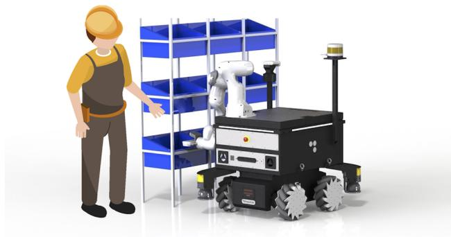
Fig. 1: A wheeled mobile manipulator and human co-worker sharing the same workspace<sup>1</sup>. In order to ensure human safety during unwanted collisions, the safety characteristics of the robot must be understood well. This work systematically investigates the safety-relevant dynamic properties of mobile manipulators for practically relevant collision scenarios in industry.
