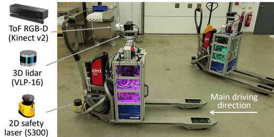
Fig. 5: Multimodal sensor setup used in our evaluation
