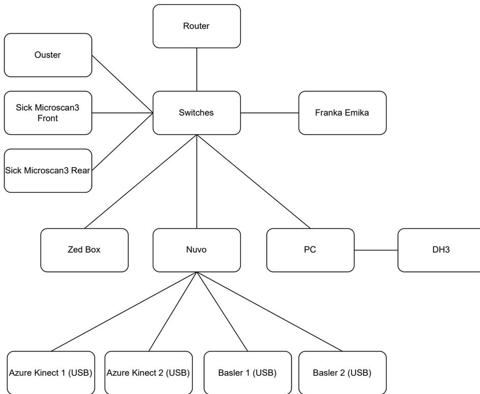
**Figure 5:** Network overview, in this chart communication network of the integrated components into the Kairos platform can be seen.
