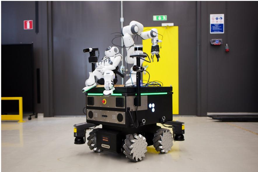
**Figure 7:** The first DARKO mobile manipulator unit (ORU) with a Nao robot on the platform
