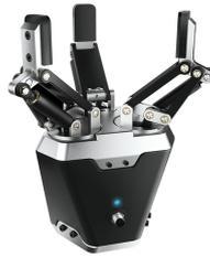
**Figure 3:** DH-3 multifinger gripper selected for the use in the first phase of the project.
