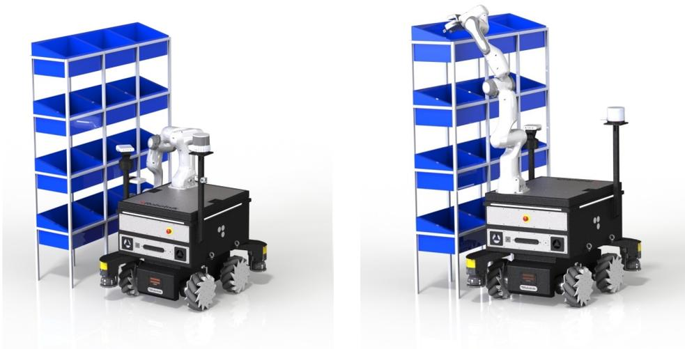
**Figure 4:** The final DARKO mobile robot equipped with the Panda robot, the gripper and the required sensors in the position of grasping objects from lower and higher shelves.
