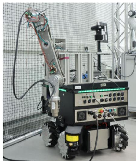
(b) TUM platform equipped with the developed elastic arm and a magnetic gripper.
