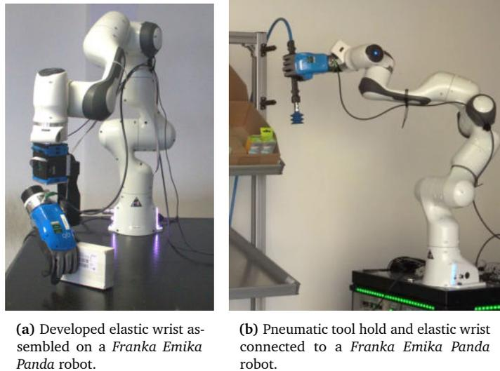
**Figure 2:** Elastic wrist and pneumatic hand-held tool developed by UNIPI. These devices, connected to the *SoftHand 2* anthropomorphic gripper, can grasp and throw various types of objects.
