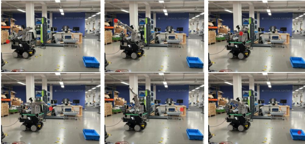
**Figure 7:** Example of throw performed by the TUM mobile manipulator equipped with the elastic arm. The location of the object at each time instant is highlighted by a red circle.
