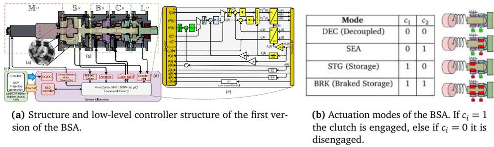
**Figure 3:** Description of the initial BSA actuator, which consists in a succession of constitutive units: Motor, Spring, Brake, Clutch and Link, and the corresponding low-level control scheme. The different states of the actuator are gathered on the table place on the right side of the figure.
