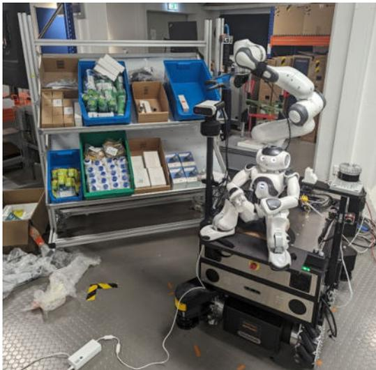
(a) ORU platform equipped with the elastic wrist during MS3.
