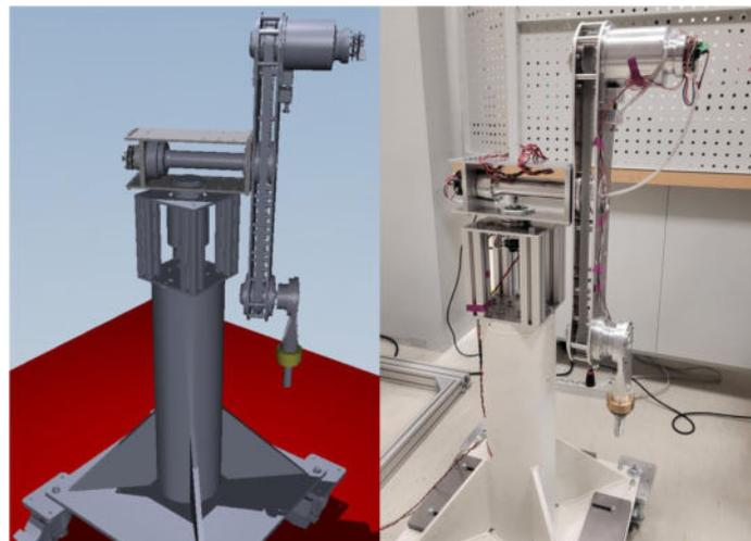
**Figure 4:** CAD representation and actual prototype of the 3-DoFs elastic arm assembled on a fixed testing structure. The 3D model on a simulation environment has been used for testing throwing control strategies, which have then been implemented on the physical prototype.
