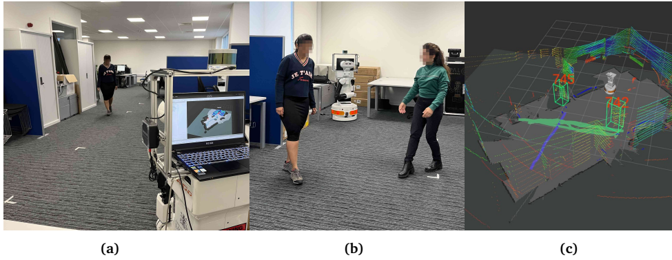
Figure 9: (a) Experimental Scenario A with two humans walking parallel to each other towards their goal (room end) and back, repetitively. The online trajectory prediction is performed by models trained on the UCY-Zara01 dataset. (b) Experimental Scenario B with two humans crossing each other's path. Here the models are trained on the THOR dataset. (c) RViz visualization of the Bayes People Tracker with human bounding-boxes extracted from the robot's LiDAR point-clouds.
